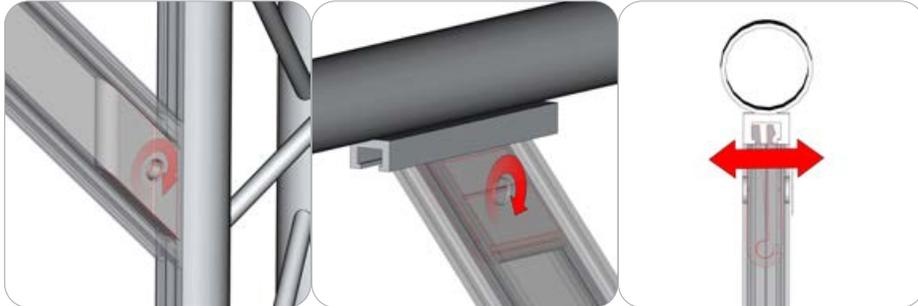
Turning counter clock-wise, use the provided allen key tool to disengage the clamp. Place the clamp teeth into the channel and turn clock-wise to engage into place. Do not over tighten.
