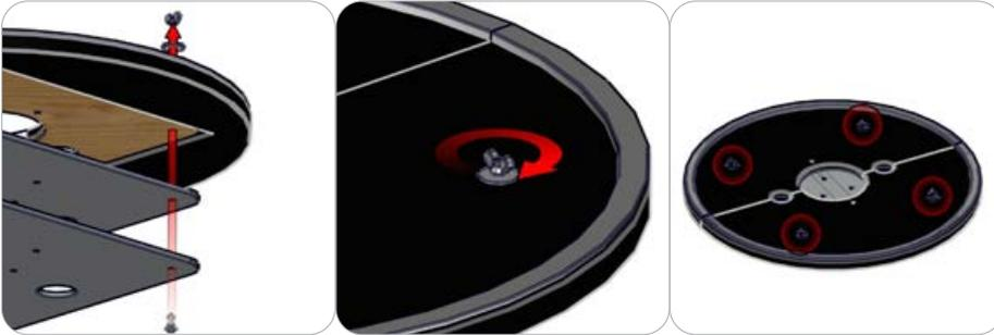
Take the two halves of the wooden round base with the two metal base plates and align them together. Use the provided hardware to fasten them together. There are four corners that you will need to fasten, each corner gets 1 bolt, 1 washer and 1 wing nut. Fasten them tight.
