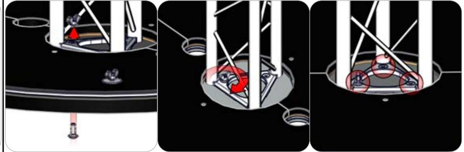
Use the provided hardware to fasten the TRI-30 on to the metal base plates. There are three holes at the end of the TRI-30, each hole gets 1 bolt and 1 washer. Fasten them tight.
