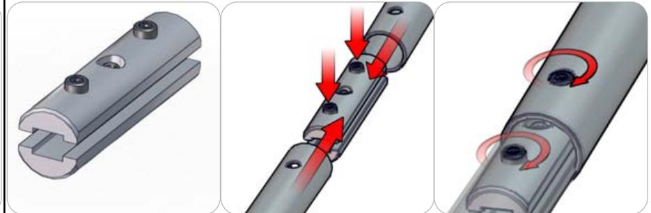
Turning counter clock-wise, loosen the screws found inside of the spigot buttons. Do not remove them. Compress the spigot and insert into the tubes. Once the spigot is in the tubes, the spigot will decompress and the button will protrude through the tubes. Turning clock-wise, lock the spigot buttons in place. Do not over tighten.
