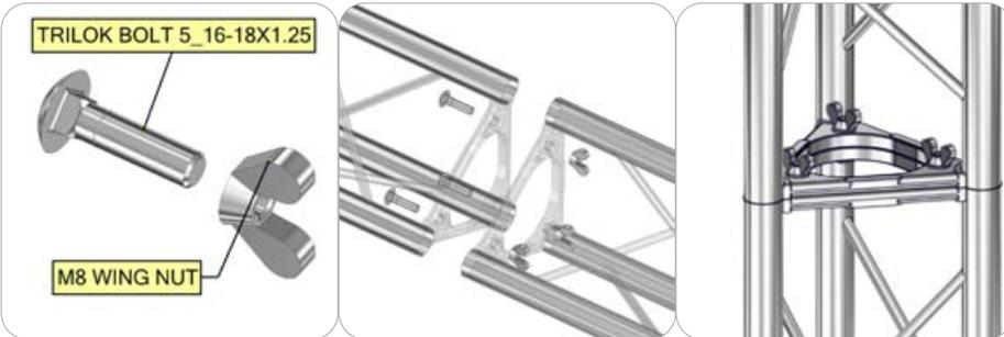
Use the provided hardware to fasten the Trilok TRI-30 to TRI-30. There are three holes to each Trilok section, each hole gets 1 bolt and 1 wing nut. Fasten them tight.
