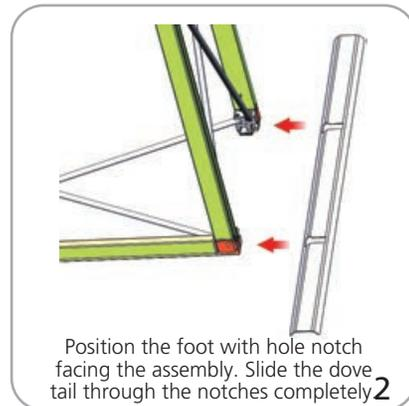
Position the foot with hole notch facing the assembly. Slide the dove tail through the notches completely. **2**
