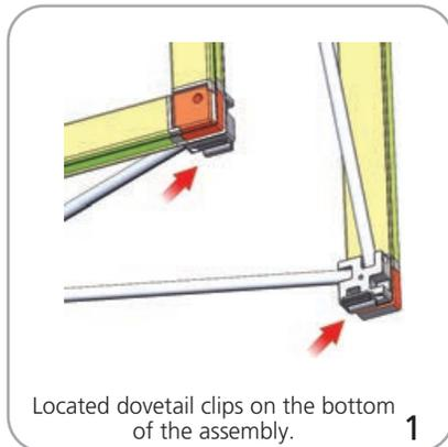
Located dovetail clips on the bottom of the assembly. **1**
