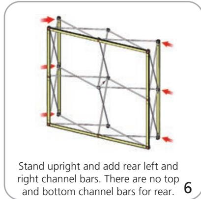
Stand upright and add rear left and right channel bars. There are no top and bottom channel bars for rear. **6**
