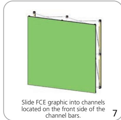
Slide FCE graphic into channels located on the front side of the channel bars. **7**
