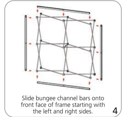
Slide bungee channel bars onto front face of frame starting with the left and right sides. **4**
