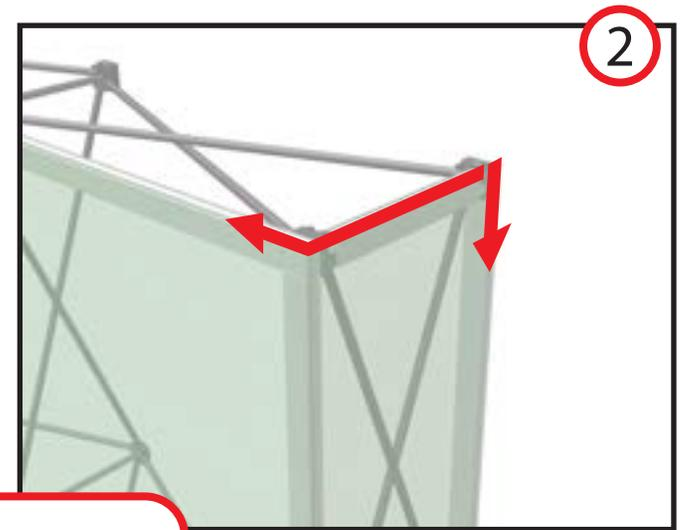
1-4. Starting in the top left corner, insert the silicone edge of the graphic into the side of the left rear channel bar and press into the groove about 6 in from the corner to secure the graphic in place. While supporting the graphic in your right hand press the silicone into the groove across the endcap channel bar and around to the front of the frame another in. While supporting the graphic move to the right side of the frame and repeat. Do this for all four corners.
