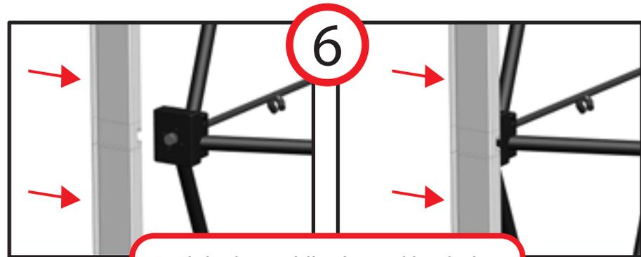
6. Slide the middle channel bar hub connector over the corresponding post of the frame hub. Push together until tight.
