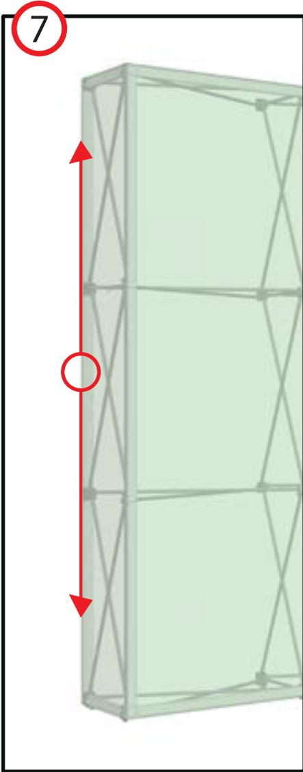
7-8. Move to the center of the left endcap and press the silicone into the SEG groove pressing the silicone into the groove alternating ether side of center until the left endcap graphic is installed. Repeat for the right endcap.
