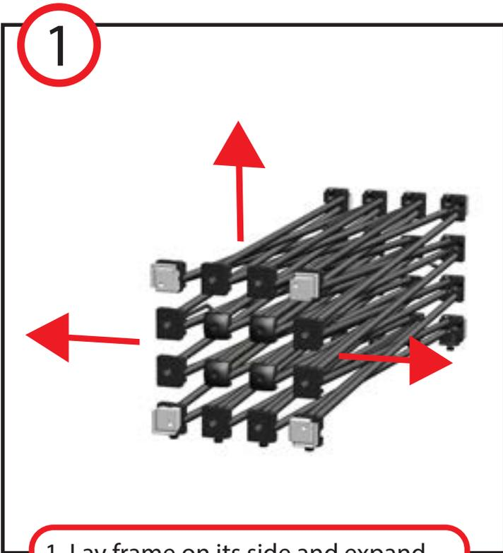
1. Lay frame on its side and expand until magnets snap into place.
