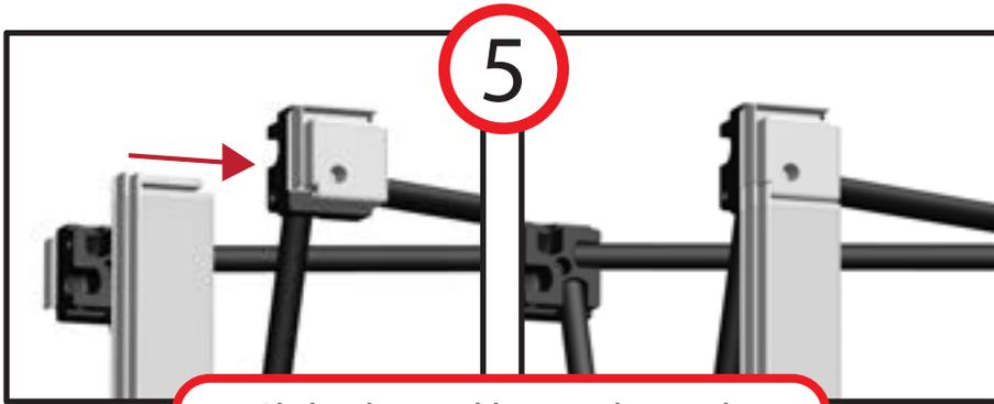
5. Slide channel bar end into the corresponding slot of the corner hub. Push together until tight.
