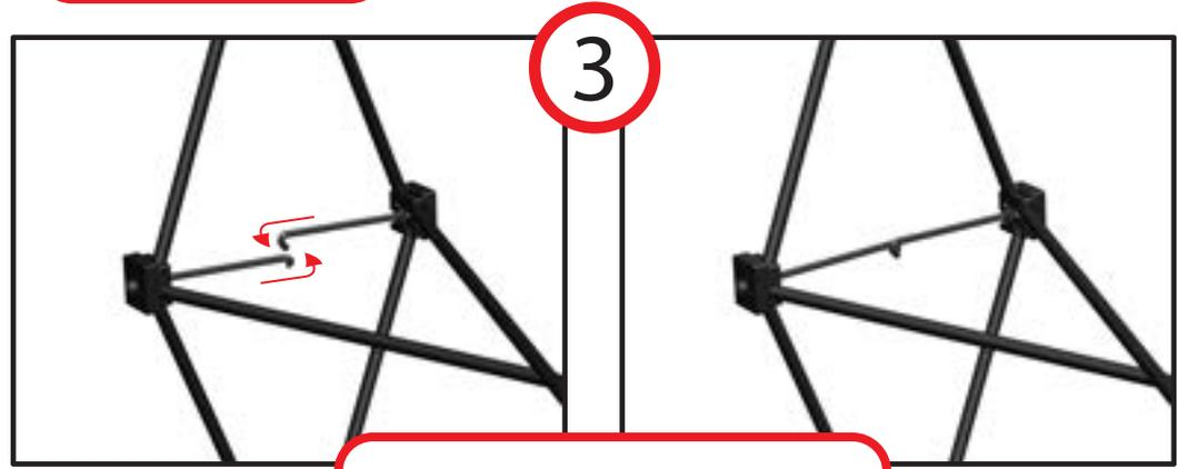
3. Attach J hooks on left and right side of frame.
